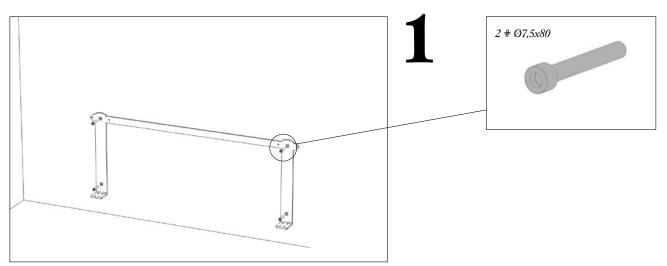
The table may only be fitted to a concrete or brick wall. Drill Ø6 mm
