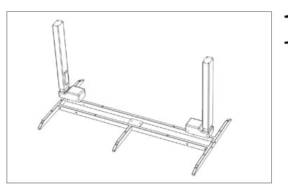
Attach the table legs to the frame by loosely screwing in all screws, before tightening (see picture 3).
